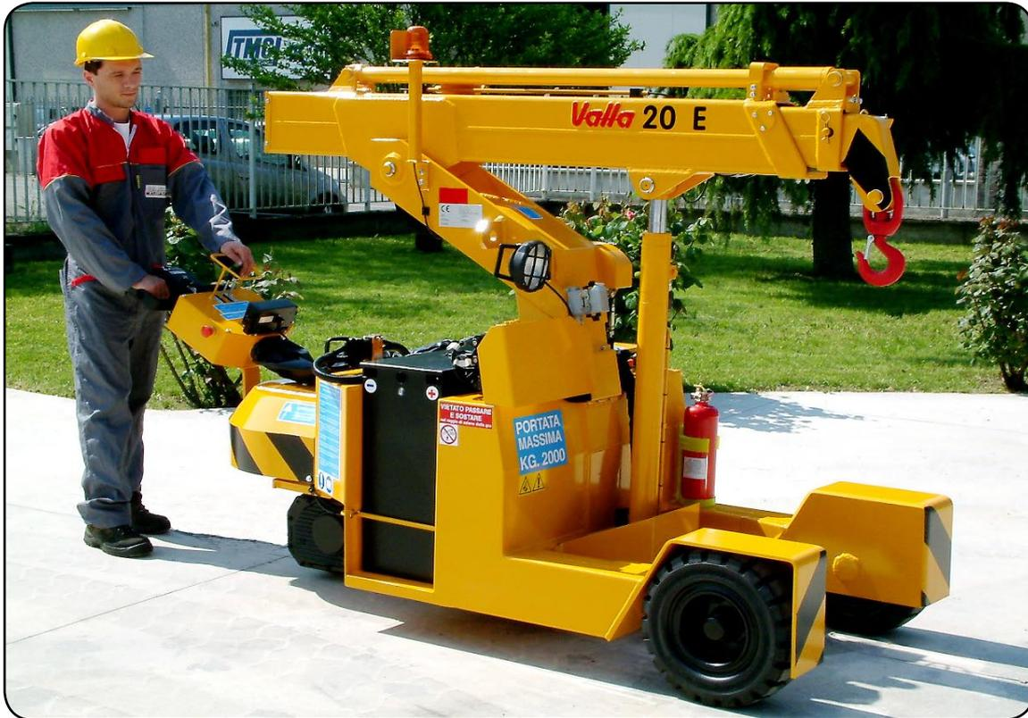
**PROPULSION:** 2 kW - 24 V AC fanned reversible electric motor fitted with electronic speed control. Disk brake on drive wheel electrically operated. Equipped with dead man cut out. Reduction between motor and wheel by gears in oil bath. Max speed 3,5 Km/h.
